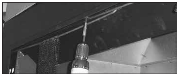
Figure 3.9 Removing the Screen Rods
