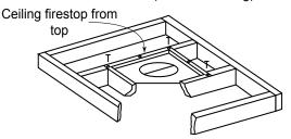
**Note:** Use same dimensional lumber for framing ceiling firestop and joists.
