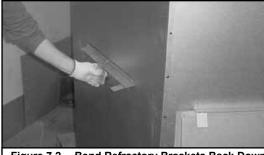
Figure 7.2 **Bend Refractory Brackets Back Down**
