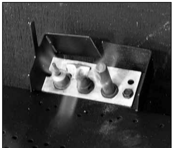
Figure 3.2 Standing Pilot Flame Patterns
