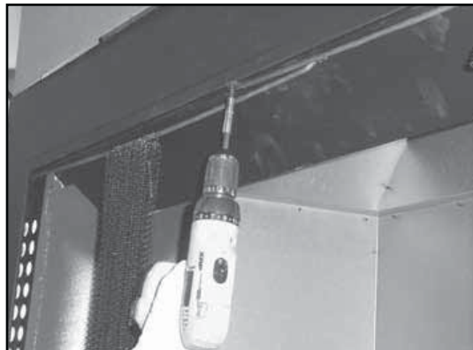
Figure 7.3 Remove Screen Rods
