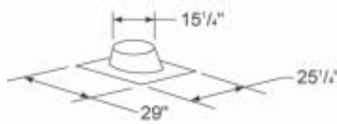
RF570 - Roof Flashing Flat to 6/12 Pitch
