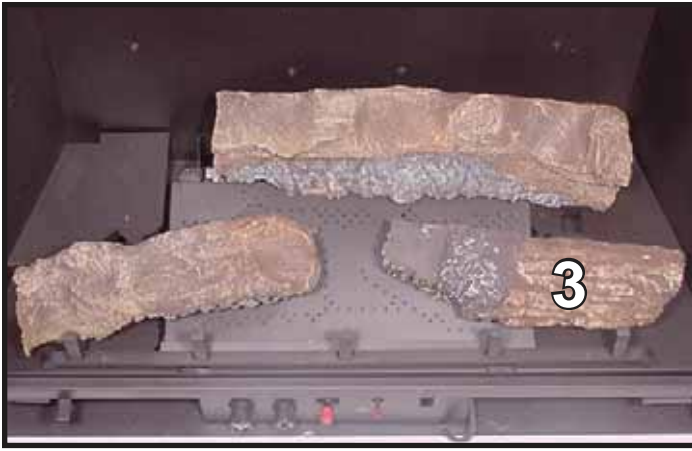
LOG #3 (SRV327-703): Position log #3 by locating its slot over the tab on the right front of the burner. The slot in the right end of log #3 fits onto the bar grate.
