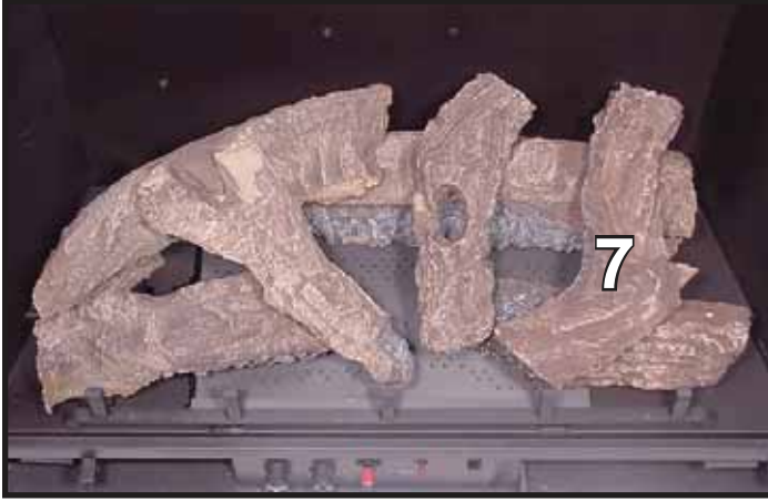
LOG #7 (SRV571-707): Rest log #7 in the smooth area just to the right of the knothole in log #1. The other end of log #7 rests on log #3 and slightly touches log #6.
