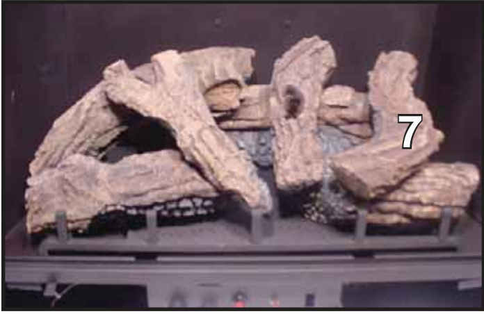
LOG #7 (SRV571-707): Rest log #7 in the smooth area just to the right of the knothole in log #1. The other end of log #7 rests on log #3 and slightly touches log #6.
