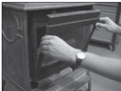
Figure 19b Removal of Sealed Glass
