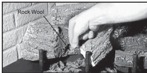
Figure 41 - Placing the Rock Wool
