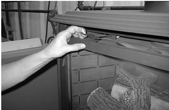
Figure 21 - Removal of Sealed Glass
