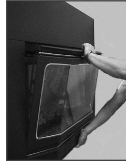
Figure 6BF Placing Bay into Slots
