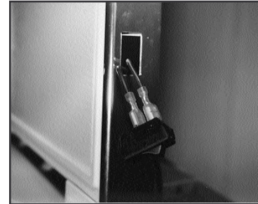
Figure 11 - Attach ON/OFF Rocker Switch Wires
