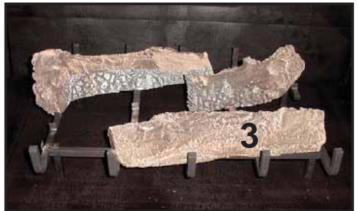
LOG #3 (SRV288-726): Position log #3 on the front right hand side of the grate against the 3 stops.
