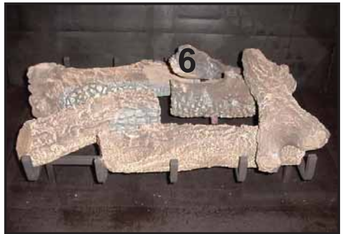
LOG #6 (SRV278-705): Place the “Y” end of log #6 over the second rear grate bend and locate its top in the locating groove on log #2.
