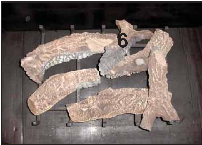
LOG #6 (SRV278-705): Place the “Y” end of log #6 over the second rear grate bend and locate its top in the locating groove on log #2.
