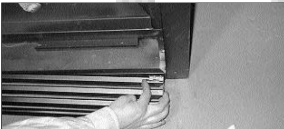
Figure 10 Lower Grille Panel Removal
