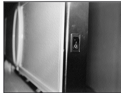
Figure 12 - "ON/OFF" Rocker Switch
