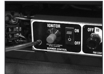
Figure 3BF Replacing Switch onto Bracket
