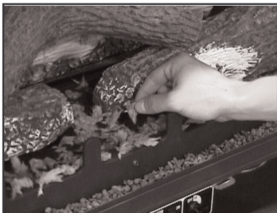
Figure 16 - Placing Rock Wool
