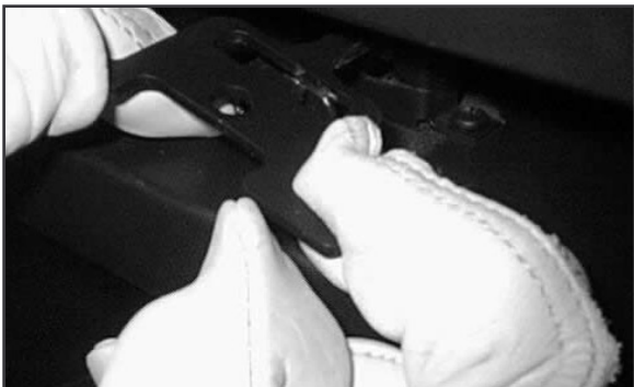
Figure 1 - Glass Retainer Latches
