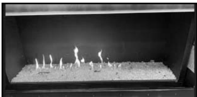
Figure 11.8 Incomplete Burner Lighting
