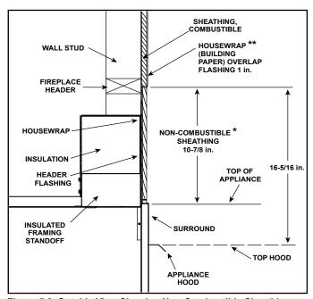
Figure 5.6 Outside View Showing Non-Combustible Sheathing
