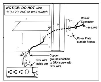
Figure 6.1 Junction Box Detail
