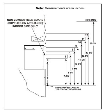
Figure 8.1 Clearances to Combustible Indoor Mantel
