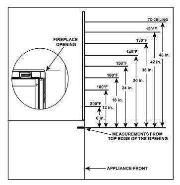
Figure 2.5 Maximum Interior Wall Surface Temperatures Above Appliance
