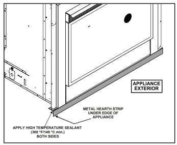
Figure 5.1 Positioning the Metal Hearth Strip
