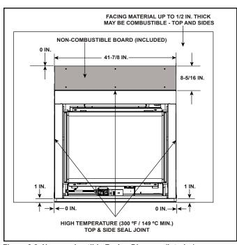
Figure 8.8 Non-combustible Facing Diagram (Interior)
