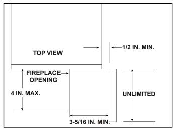
Figure 8.4 Clearances to Non-Combustible Indoor Mantel or Mantel Leg
