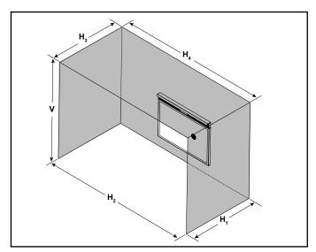
Figure 2.3 Three Sided Enclosure Example
