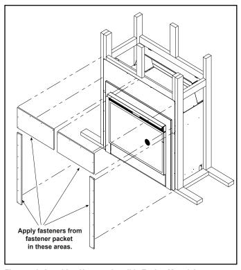
Figure 5.8 Attaching Non-combustible Facing Material (Outdoor Side Only)
