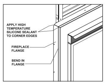
Figure 5.3 Application of High Temperature Sealant
