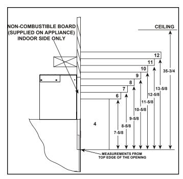
Figure 8.2 Clearances to Non-combustible Indoor Mantel
