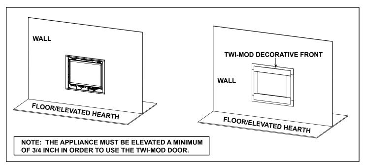
Figure 8.5 Appliance Installed Off the Floor
