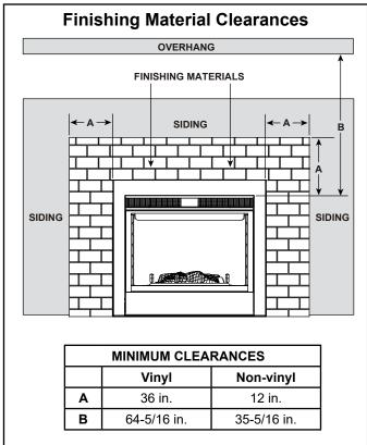
Figure 3.4 Exterior View - Finishing Material Clearances
