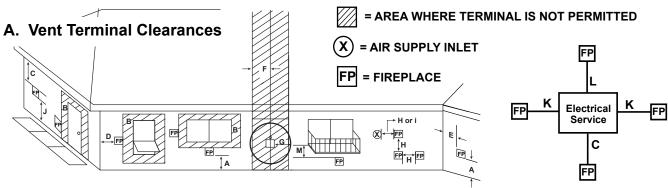
**U.S.A.** Installations: In accordance with the current ANSI Z223.1/NFPA 54, National Fuel Gas Code. Canadian Installations: In accordance with the current CSA B149.1, Natural Gas and Propane Installation Code.
