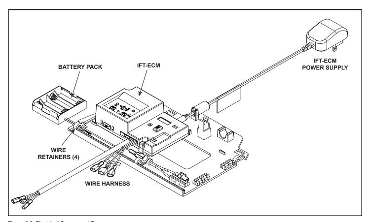
Figure 6.2 Electrical Component Tray
