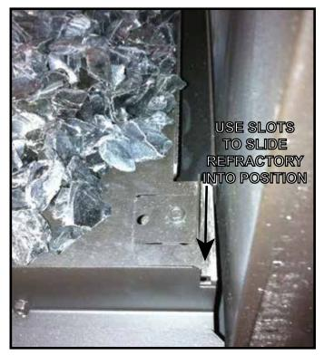
Figure 9.7 Install Refractory
