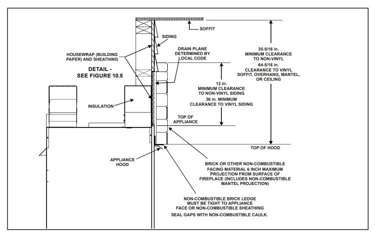
Figure 8.13 Exterior View with Non-combustible Facing Material
