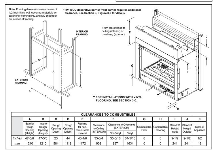
Figure 3.3 Clearances to Combustibles
