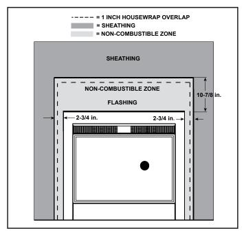
Figure 5.7 Exterior Installation Prior to Finishing
