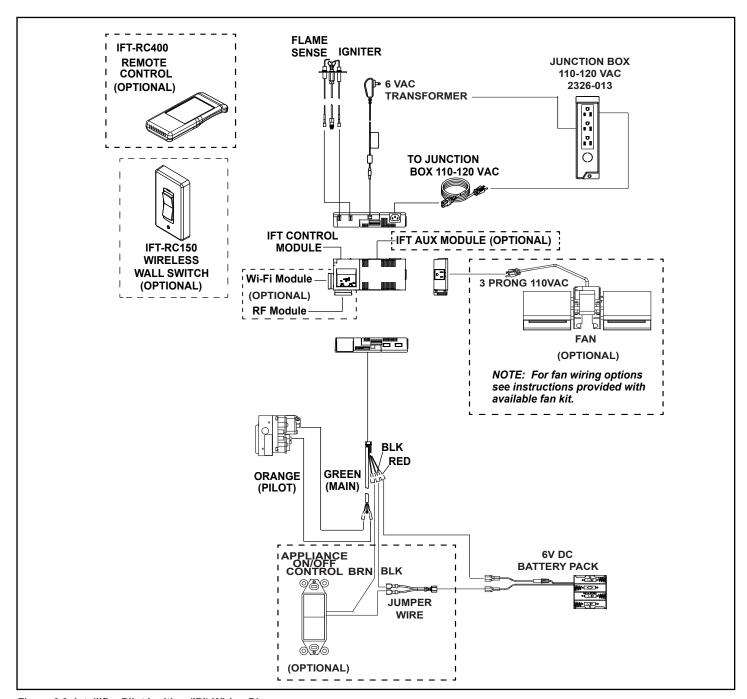
Figure 6.3 Intellifire Pilot Ignition (IPI) Wiring Diagram
