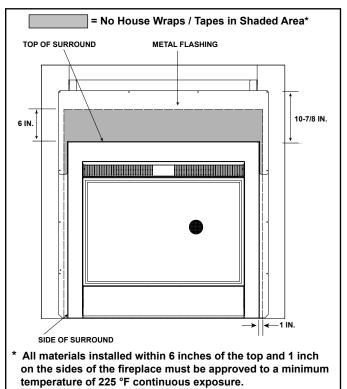
Figure 5.5 Outside View without Non-Combustible Sheathing Shown
