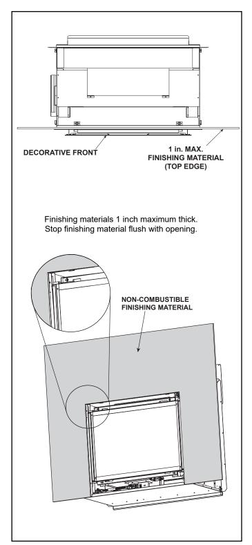
Figure 8.10 Finishing Material 1 Inch Thick or Less
