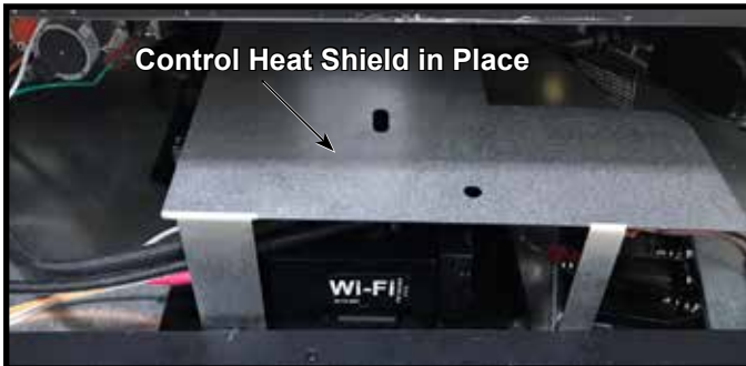
Figure 11.2 Control Heat Shield - Installed
