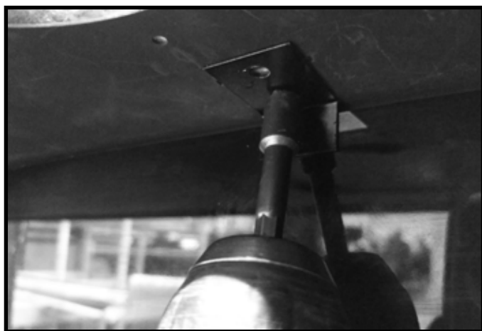
Figure 3 Retaining Bracket Installation - Back
