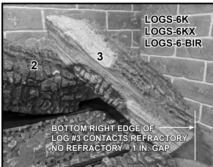
Figure 5.B Place Log #3 (LOGS-6K / LOGS-6KX / LOGS-6-BIR)
