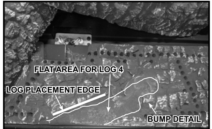
Figure 8 Log Placement Details
