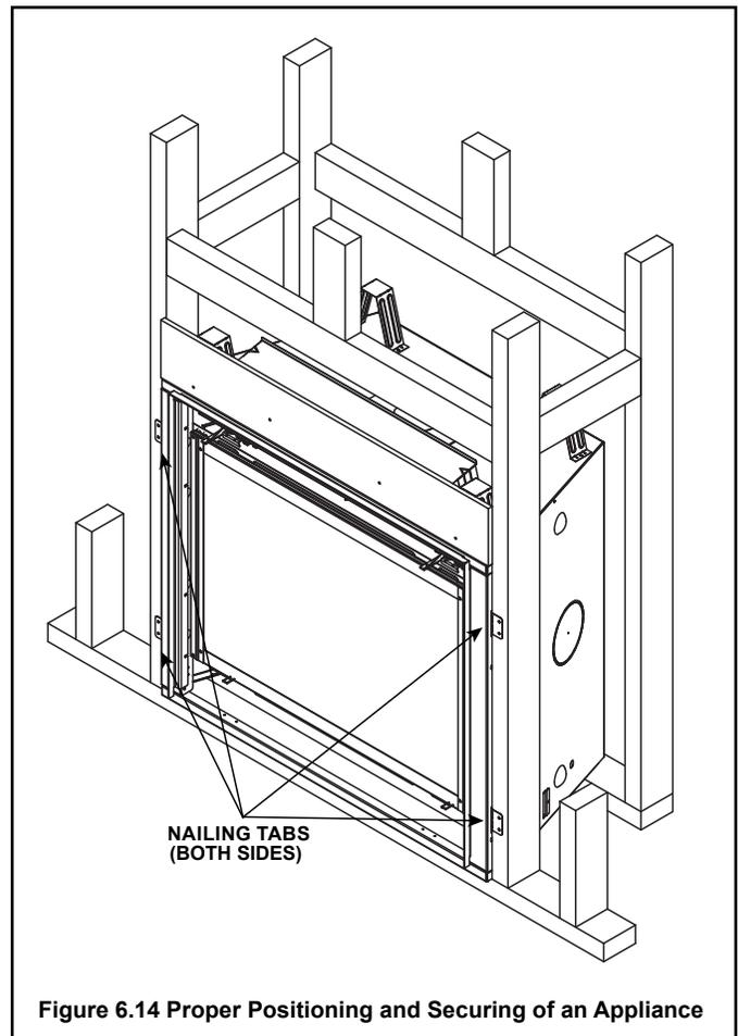
Figure 6.14 Proper Positioning and Securing of an Appliance
