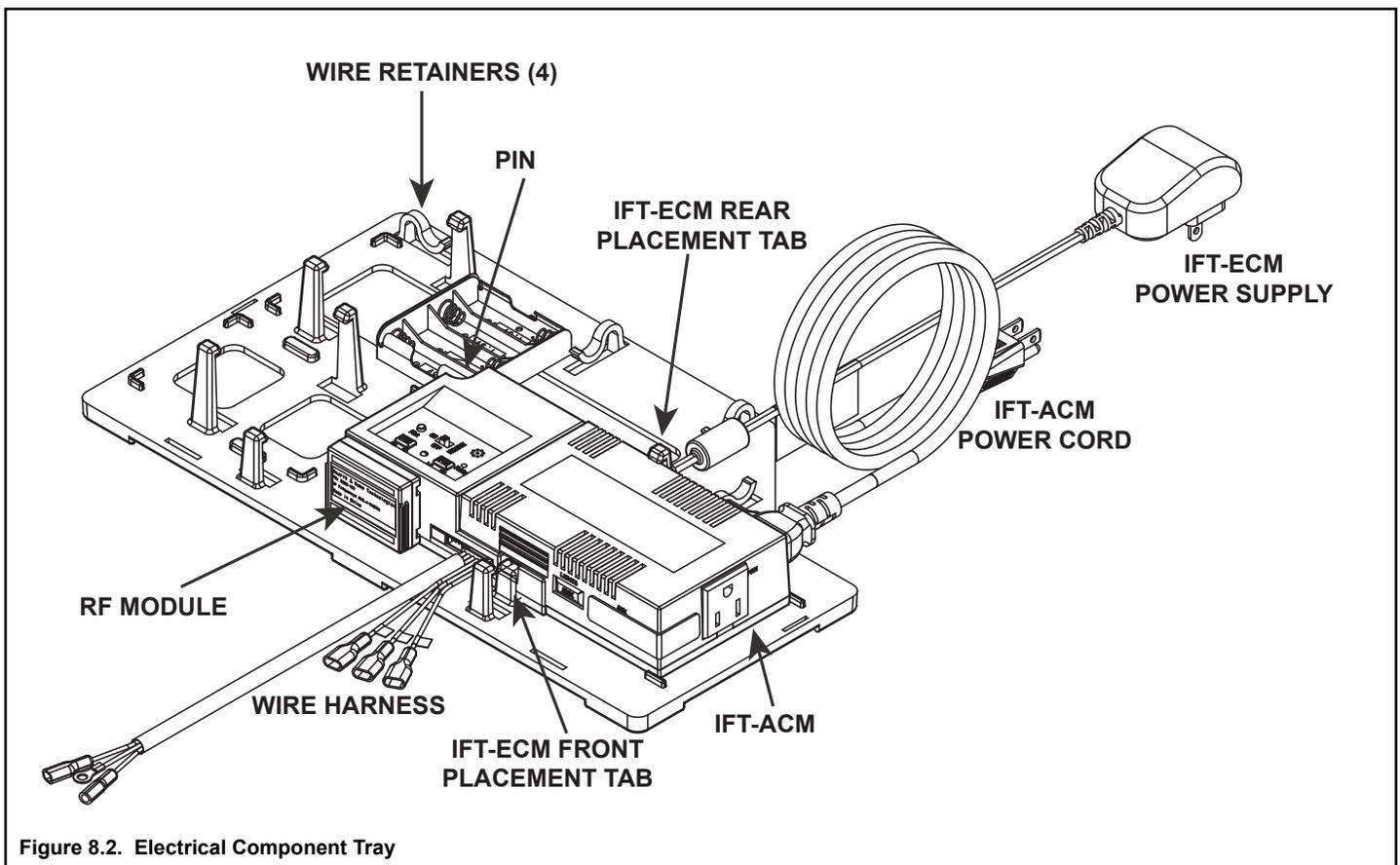
Figure 8.2. Electrical Component Tray
