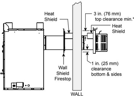
\* When using SLP pipe, minimum clearances from the vent pipe to combustible materials at inside wall firestops are:
