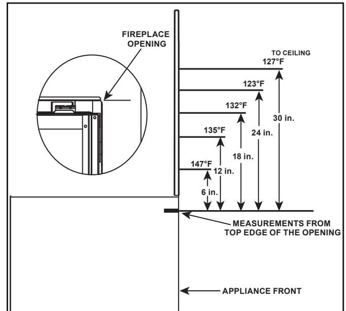
Figure 2.1 Good Faith Wall Surface Temperatures Above Appliance
