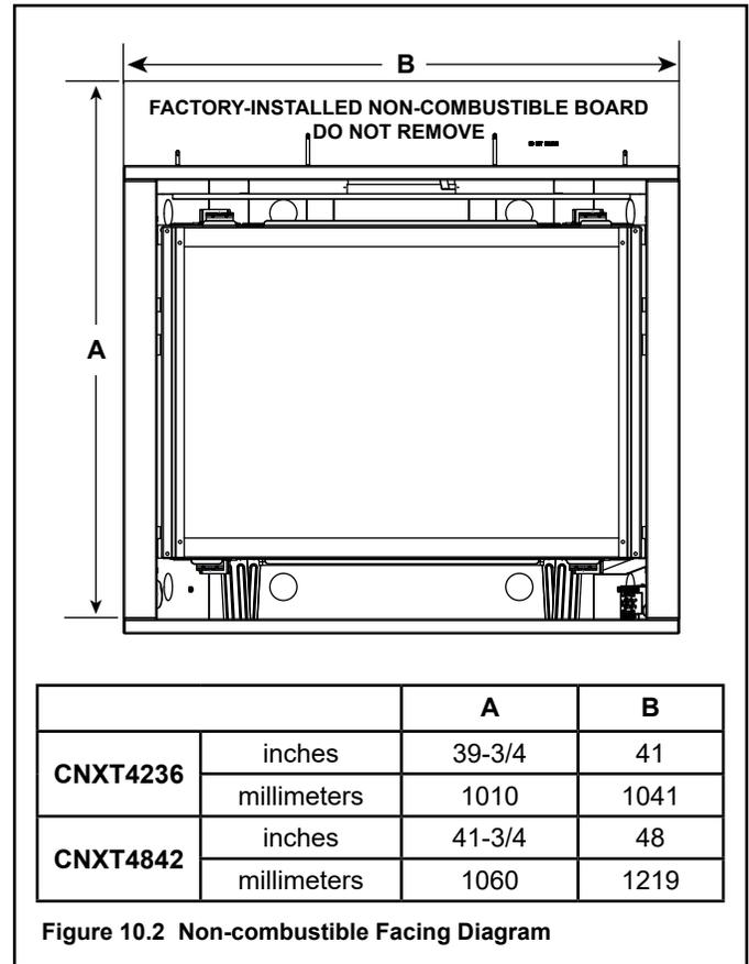
Figure 10.2 Non-combustible Facing Diagram
