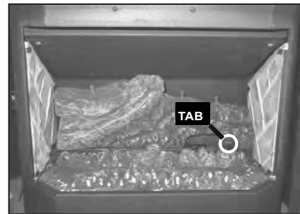
Figure 8.7 Insert rear log (#1) onto log pan over stud on the left, gently pulling log forward to the tab on the right.
