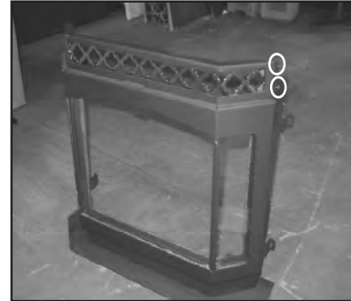
Figure 8.2 To remove the original grille, loosen the four screws from the left and right sides at the top of the door. Slide grille off, remove the screws and set aside. Discard the original grille.
