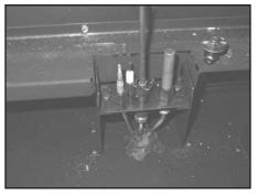
**Figure 6.4** Remove the pilot hood, and set aside. Using a 5/32 in. allen wrench, remove the pilot injector and replace with an appropriate injector (35 LP, 62 NG).
