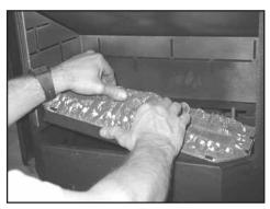
Figure 6.2 Lift the burner from the left side and slide left until free from the orifice receiver. Remove from the firebox and handle with care.
