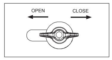
**Figure 8.14** The shutter is located on the underside of the appliance, on the right side. To adjust the shutter, loosen the wingnut.. Retighten the wingnut after adjustment.
