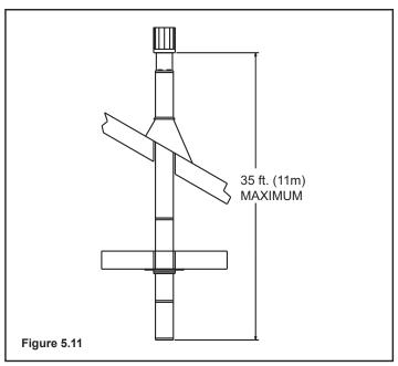
NOTE: Maximum number of 90° elbows permitted for a vertical installation is four, provided the termination falls within the shaded area shown in vent graph on page 10. See also **Figure 5.12**, within the four 90° elbows configuration, the maximum allowable pipe length on the horizontal runs is 1 ft. (305mm) the minimum allowable pipe length on vertical runs is 1 ft. (305mm).
