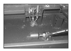
**Figure 6.3** With a 5/8 in. wrench remove orifice retaining nut. Replace with appropriate orifice.
