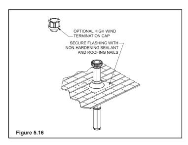
**Step 9.** Twist-lock the vent cap and seal.
