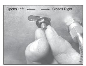
Figure 6.1 Loosen the shutter adjustment nut (located underneath the appliance) with a 7/16 in. wrench.
