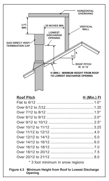
**Figure 4.3** specifies minimum vent heights for various pitched roofs.
