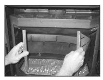
**Figure 8.4** Holding both sides of the metal refractory brick piece, pull slightly together and rotate out of the firebox.
