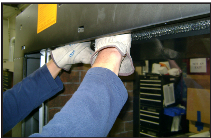
Figure 11.6 Top Glass Latch Access
