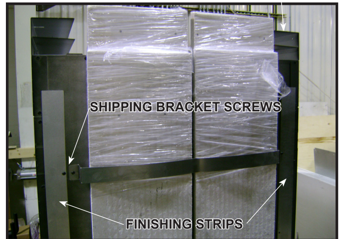
Figure 6.3 Shipping Brackets and Finishing Strip Locations.
