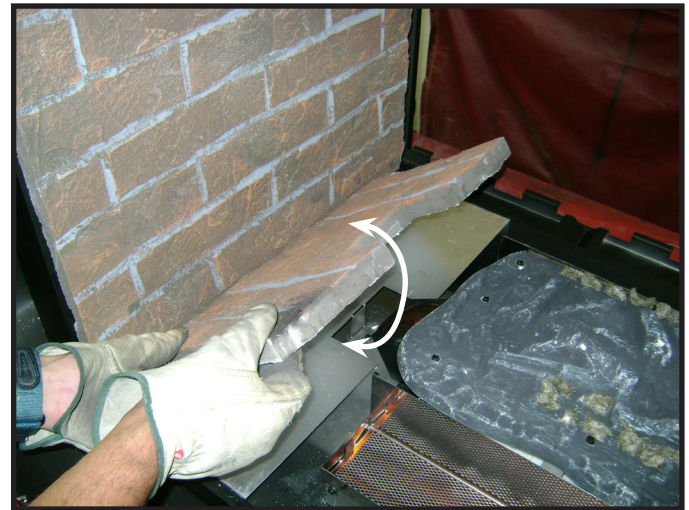
Figure 11.17 Positioning Inner Bottom Refractory
