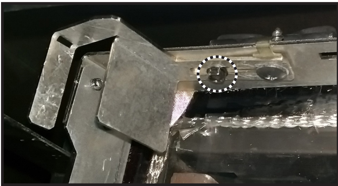
Figure 11.26 Shipping Location of Refractory Brackets
