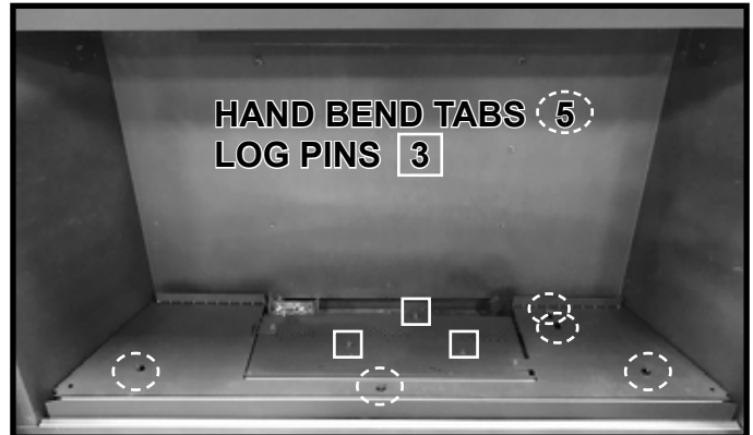
Figure 3. Hand Bend Tab and Log Pin Locations
