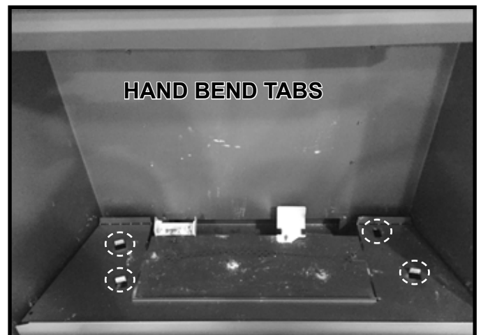
Figure 3. Hand Bend Tab Locations - QUARTZ36 Shown
