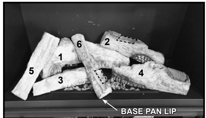
Figure 11. Install Middle Left Cross Log
