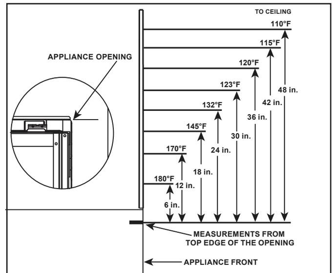
Figure 3.3. Maximum Wall Surface Temperatures Above Appliance
