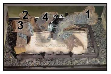
STEP 5. LOG #4 (SRV2005-703): Locate the sharp notch on log #4 against the grate tine as shown. The smooth cutout on the bottom of log #4 should rest on the burner surface. The side of Log #4 must be 3/4 inch from the nearest port hole on the right side of log #4. **DO NOT** cover any port holes.
