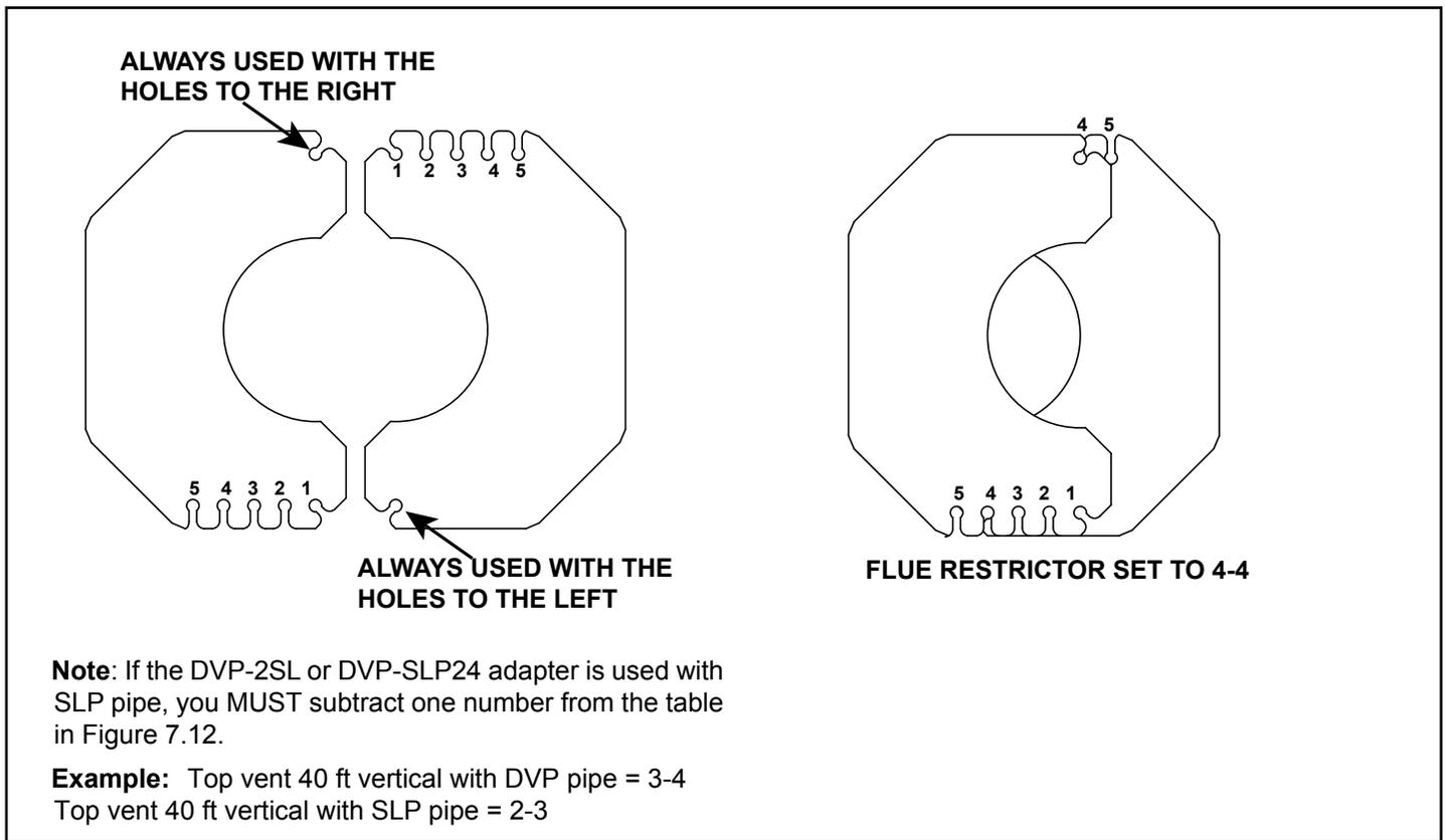
Figure 7.13. Setting the Flue Restrictor
