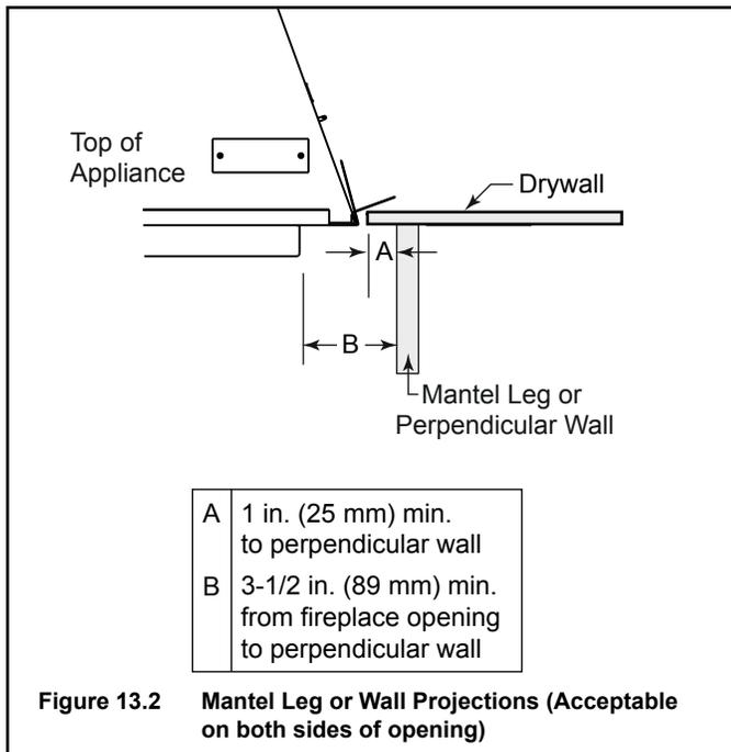
Figure 13.2 Mantel Leg or Wall Projections (Acceptable on both sides of opening)
