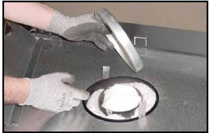
**Figure 9.3** Remove the seal cap.
