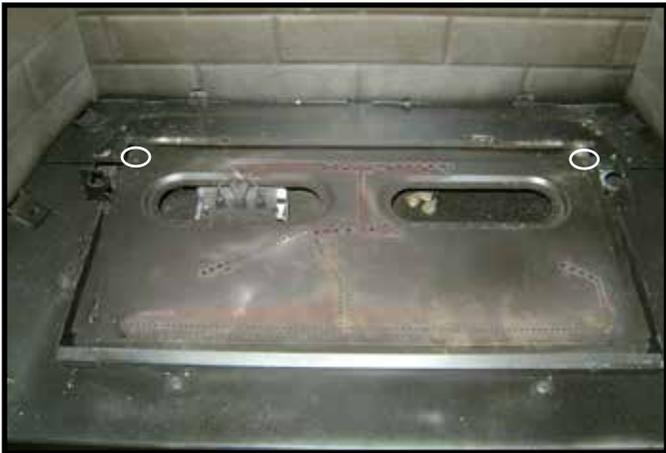
Figure 3.8 Remove Screws from Burner Assembly Rear Corners
