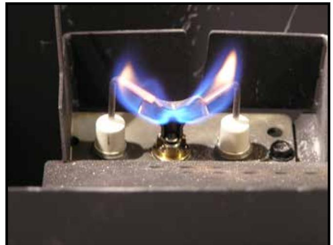
Figure 3.1 IPI Pilot Flame Patterns
