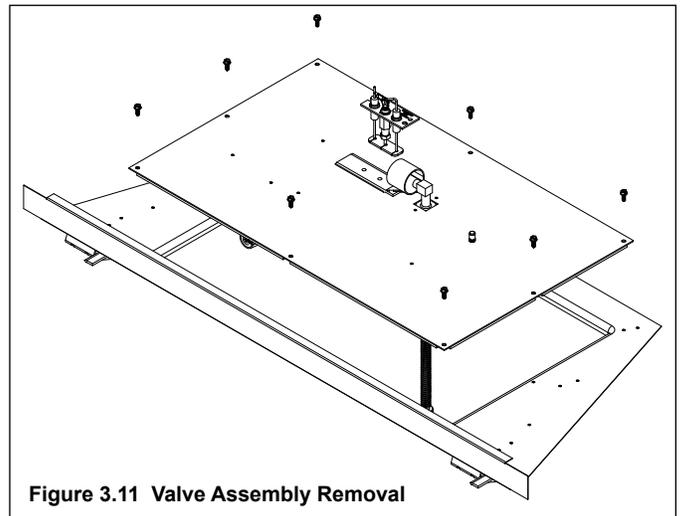
Figure 3.11 Valve Assembly Removal
