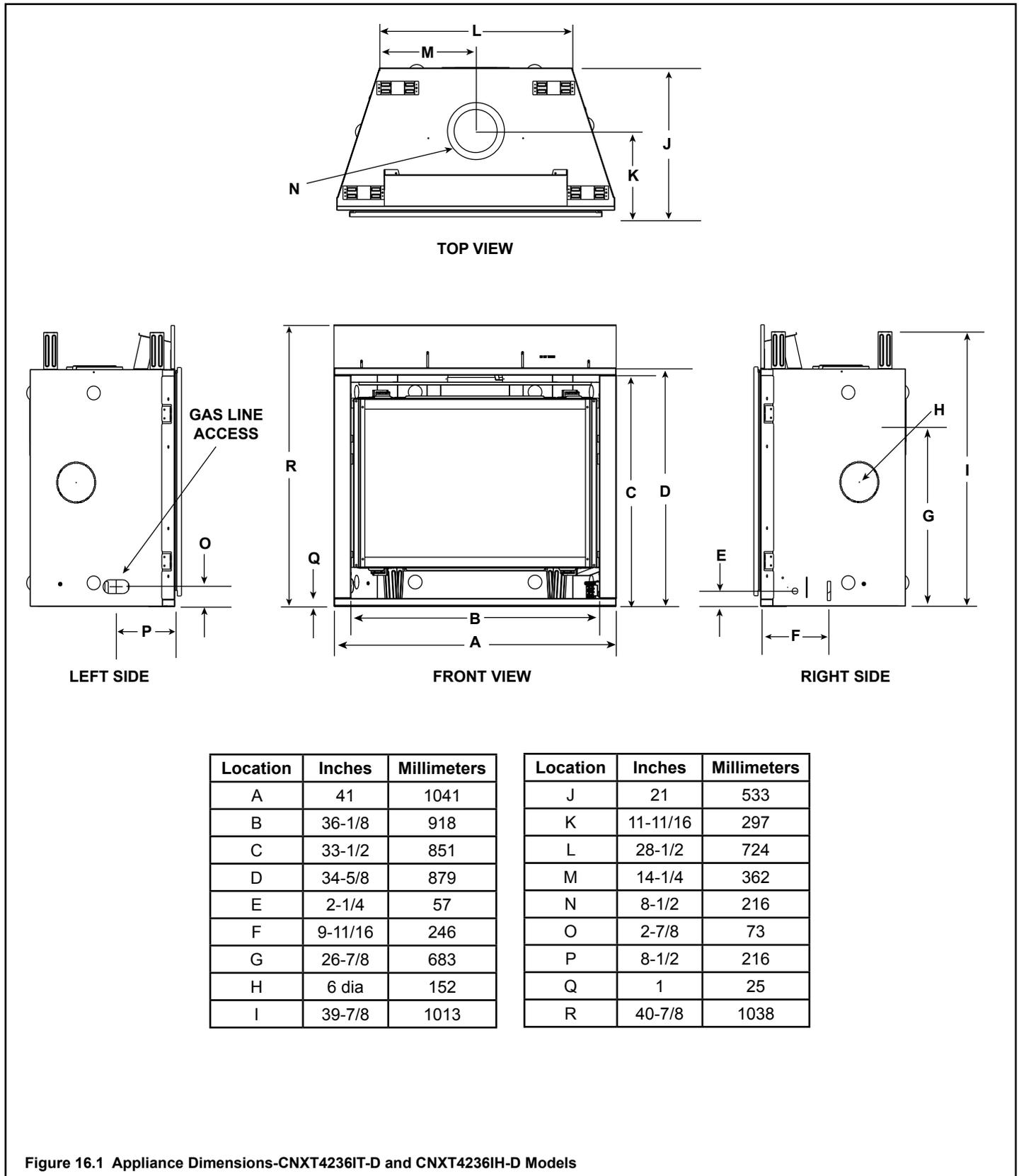
Figure 16.1 Appliance Dimensions-CNXT4236IT-D and CNXT4236IH-D Models
