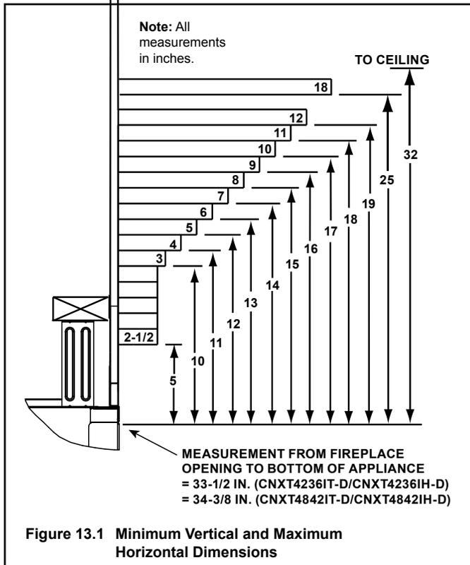
Figure 13.1 Minimum Vertical and Maximum Horizontal Dimensions
