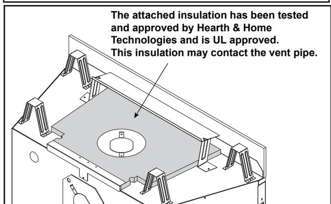
➔ **Figure 8.2 CNXT4842IT-D, CNXT4842IH-D Top Insulation**
