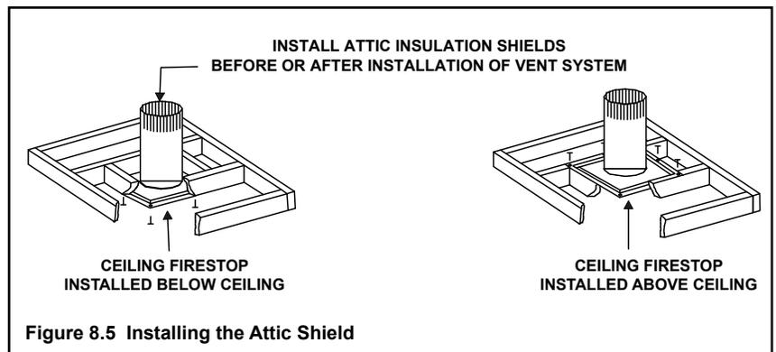
Figure 8.5 Installing the Attic Shield
