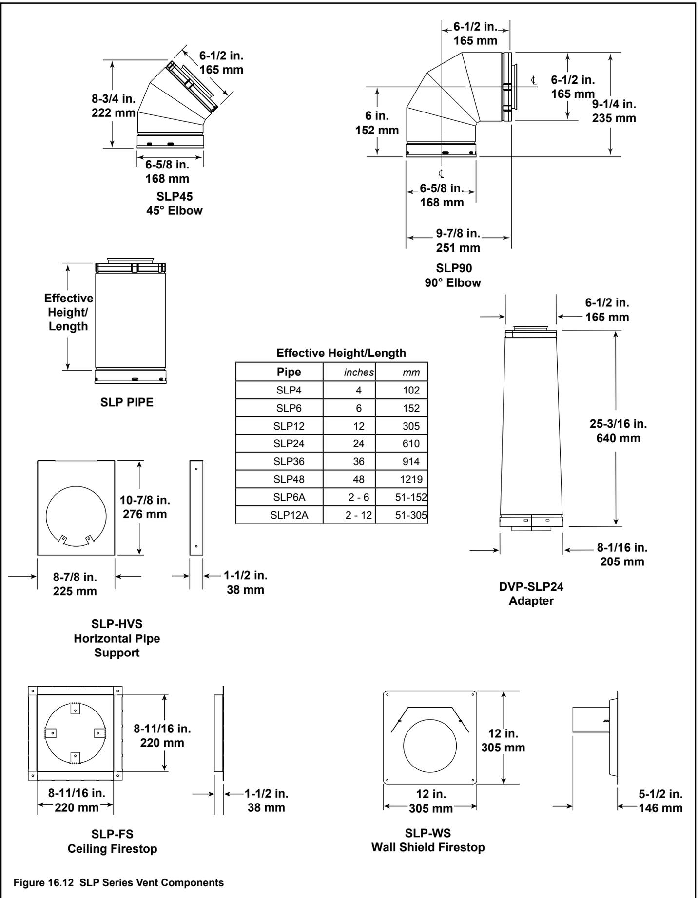
Figure 16.12 SLP Series Vent Components
