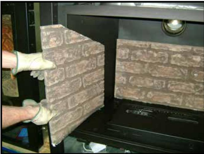
Figure 3.3 Side Refractory Removal
