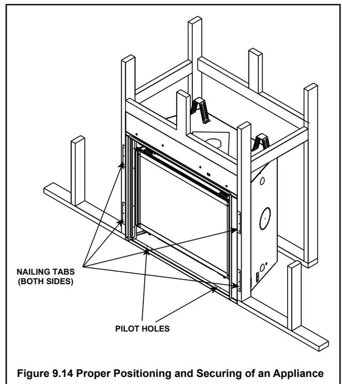
**Figure 9.14** Proper Positioning and Securing of an Appliance
