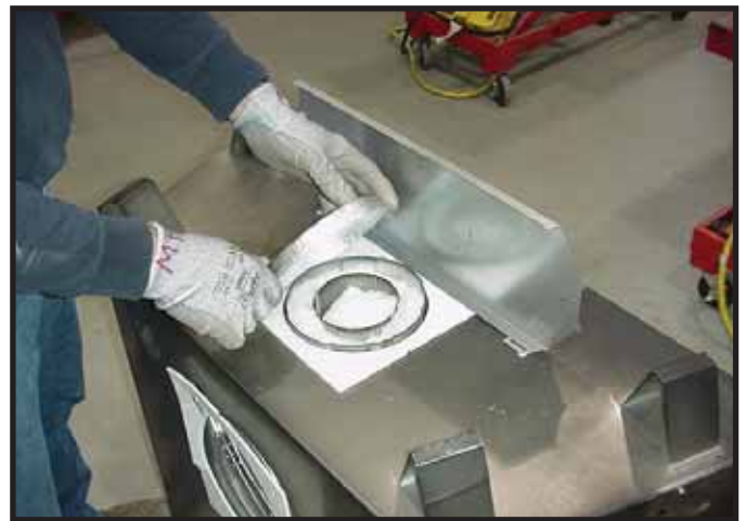
Figure 6.4 Remove the seal cap.
