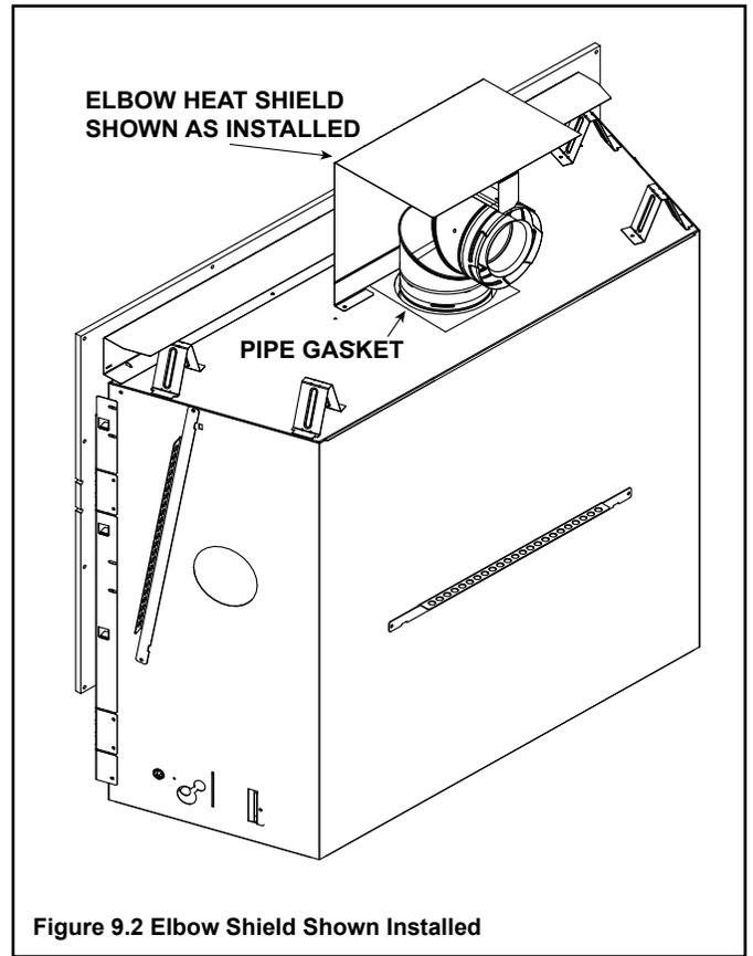
If venting with a 90 degree elbow directly off of the top of the appliance, the elbow heat shield must be repositioned as shown in Figure 9.2.
