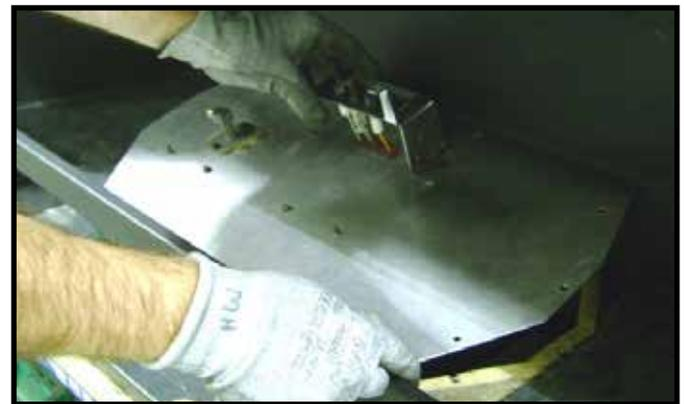
Figure 11.3. Remove Valve Plate
