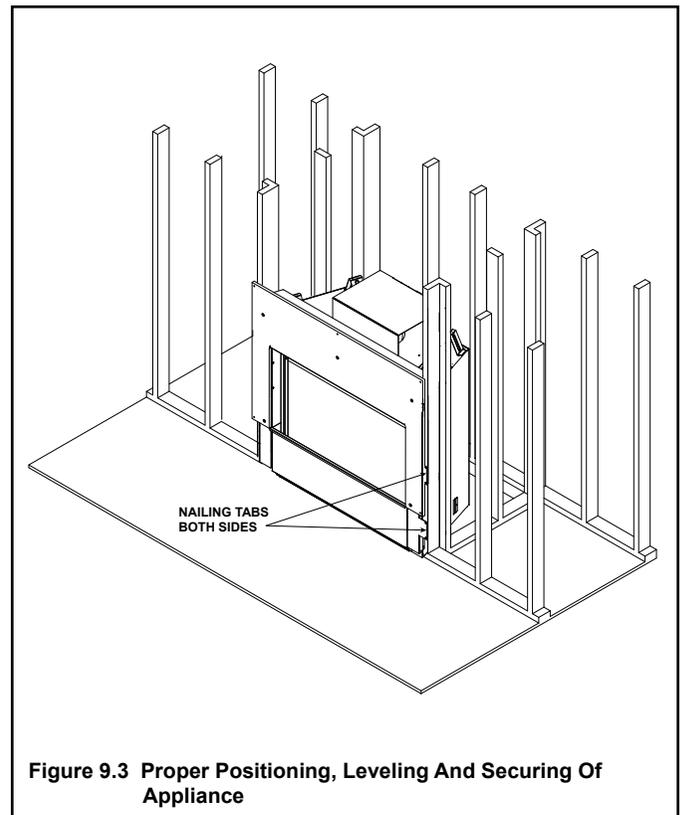
**Figure 9.3 Proper Positioning, Leveling And Securing Of Appliance**
