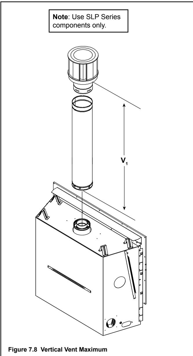
Exhaust restrictors are recommended for these vertically terminated products which have excessive draft. Exhaust restrictors will compensate for high draft, and restore visual flame height. If the vent configuration has a total vertical of 15-44 feet, an exhaust restrictor may be needed. The exhaust restrictor can be located in the appliance manual bag.
