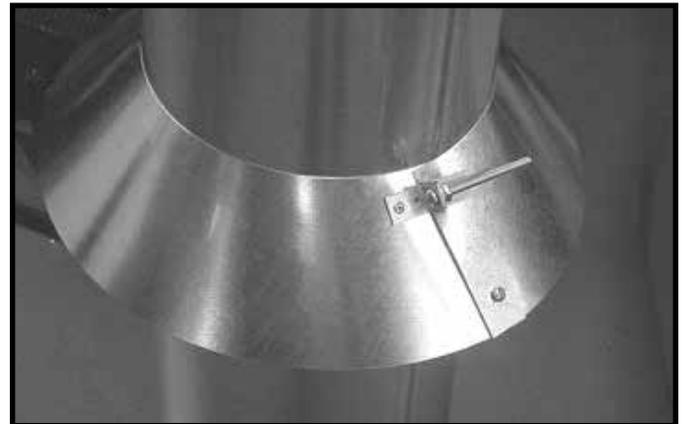
**Figure 10.13 Assembling the Storm Collar Around the Pipe**
