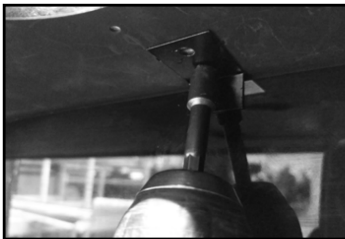
Figure 3 Retaining Bracket Installation - Back
