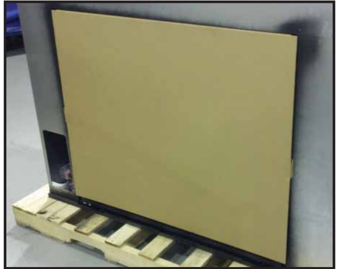
Figure 13.5. Splatter Guard Installation
