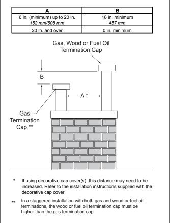
Figure 6.2 Staggered Termination Caps
