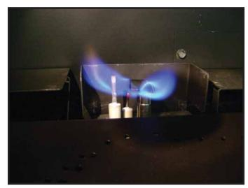
Figure 3.2 IPI Pilot Flame Patterns
