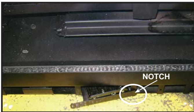
Figure 2.4 Pull Left Side of Tray Out and Disengage Notch
