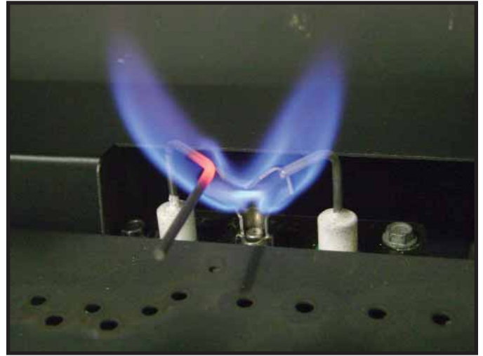
Figure 3.1 IPI Pilot Flame Patterns
