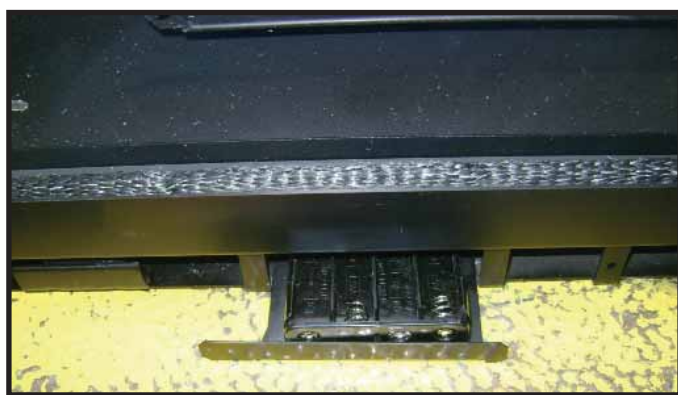
Figure 2.5 Battery Tray Pulled Out
