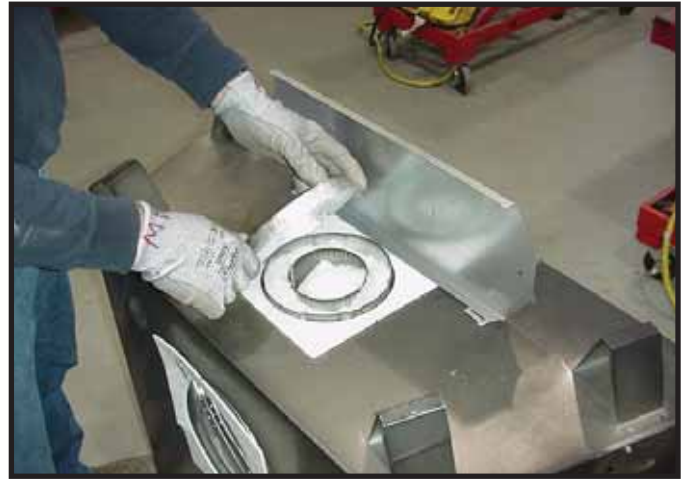
Figure 9.4 Remove the seal cap.
