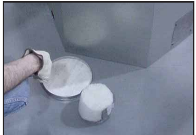
Figure 9.11 Discard the seal cap, remove and discard the insulation basket. Note: Once the seal cap has been removed it CANNOT be reattached.
