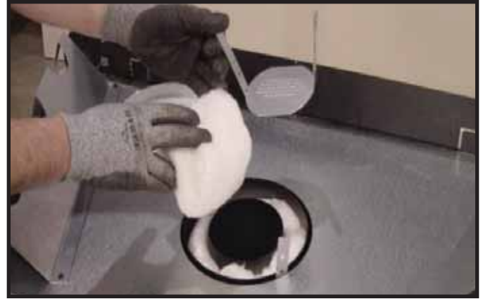
Figure 9.4 Remove the insulation basket and white insulation from the center vent pipe.
