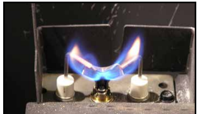
Figure 3.1 IPI Pilot Flame Patterns
