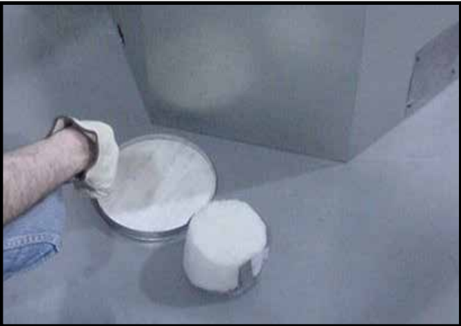
Figure 9.15 Discard the seal cap, remove and discard the insulation basket. Note: Once the vent cap has been removed it CANNOT be reattached.
