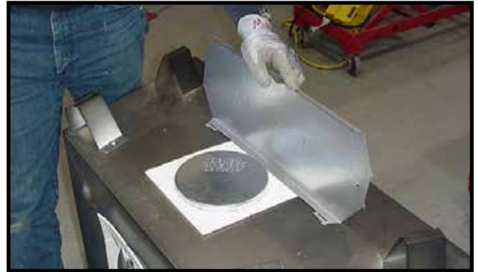
Figure 9.4 Rotate the top heat shield to the vertical position as shown above. The heat shield must remain in the vertical position.
