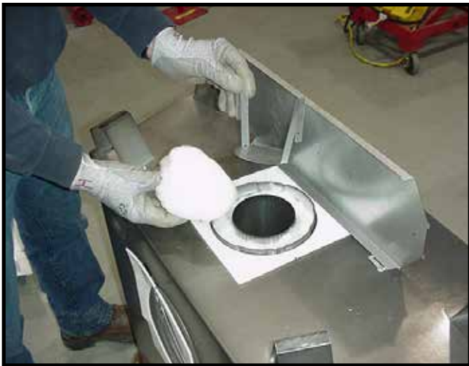
Figure 9.7 Remove the insulation basket and white insulation from the center vent pipe.
