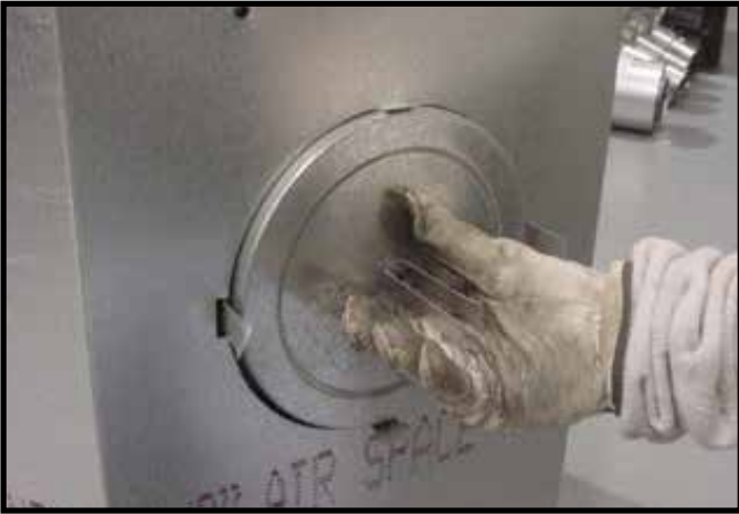
Figure 9.14 Fold the center parts of the retaining band out and use to remove the seal cap.
