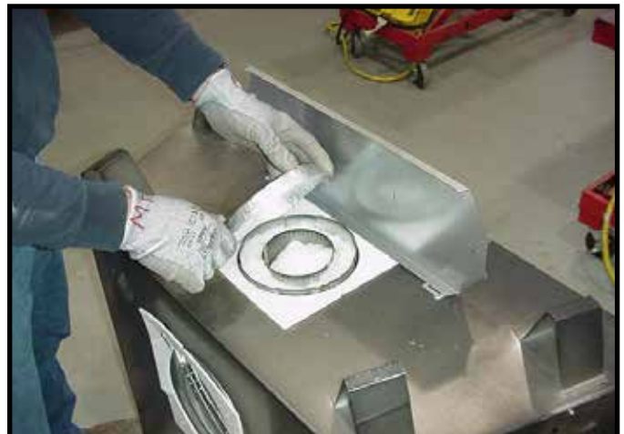
Figure 9.6 Remove the seal cap.
