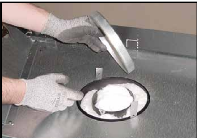
Figure 9.3 Remove the seal cap.
