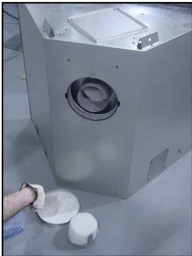
Figure 9.10 Discard the vent cap, remove and discard the insulation basket.
