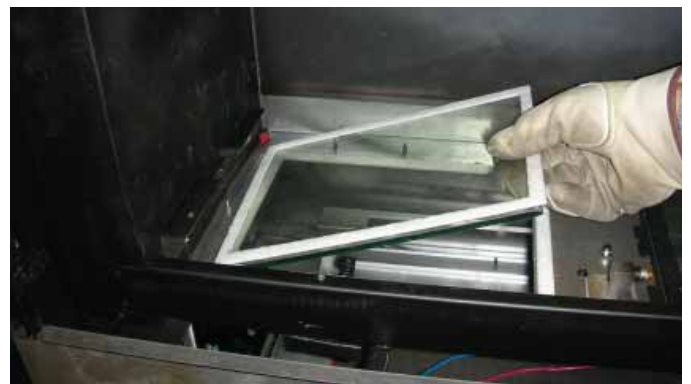
Figure 8.13 Removing Glass Pane Frame
