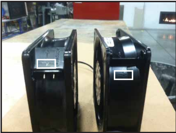
Figure 8.20. Arrow Indicates Direction of Air Flow
