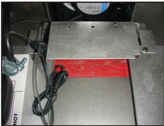
Figure 8.15 Blower Mounting Bracket
