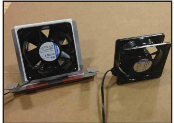
Figure 8.21. Proper Blower Mounting.
