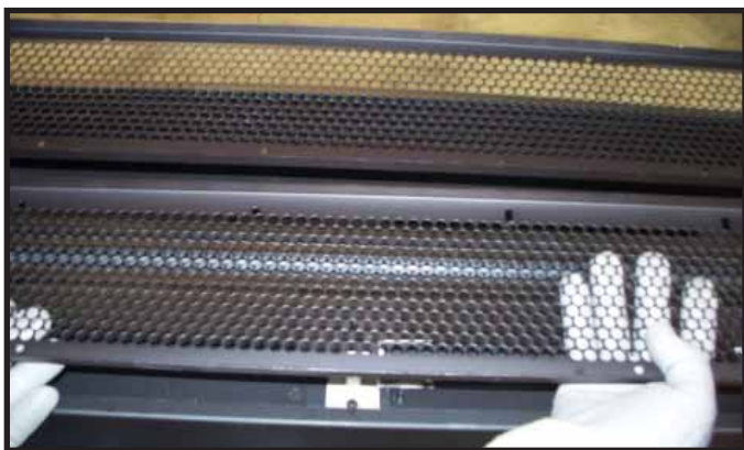
Figure 8.10 Lifting Base Pan Up and Out.
