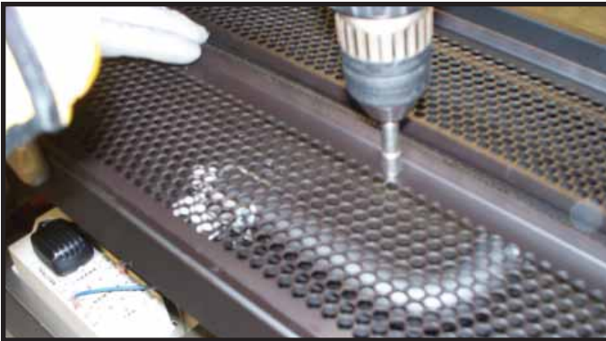
Figure 8.9 Removing Screws from Base Pan
