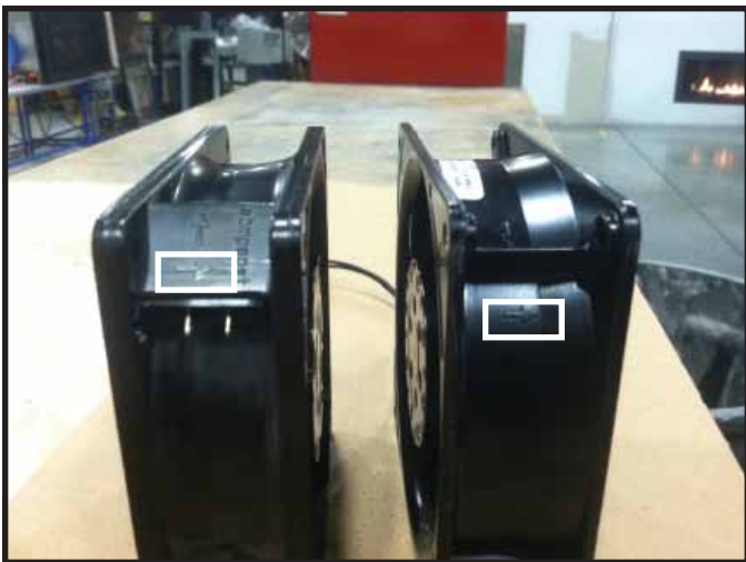
Figure 8.20. Arrow Indicates Direction of Air Flow
