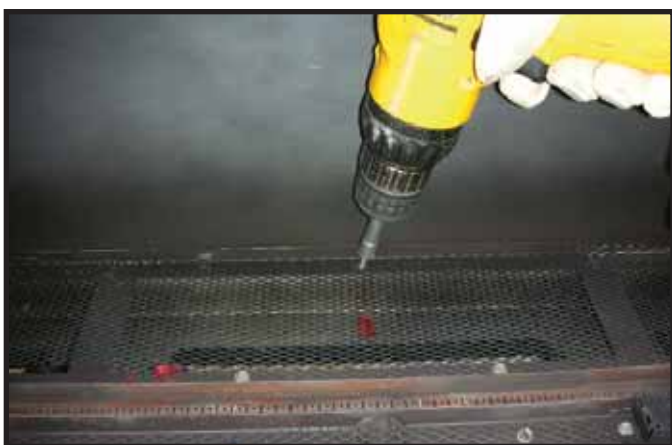
Figure 5. Removing Screws from Basepan.
