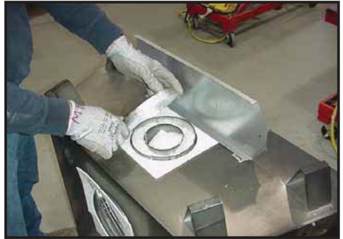
Figure 9.4 Remove the seal cap.
