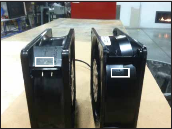
Figure 8.20. Arrow Indicates Direction of Air Flow
