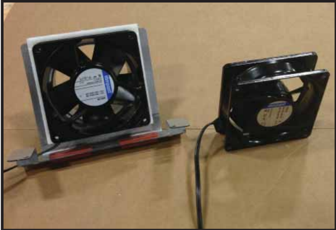
Figure 8.21. Proper Blower Mounting.
