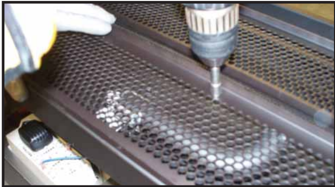
Figure 8.9 Removing Screws from Base Pan.
