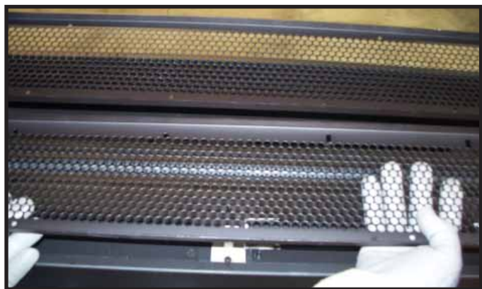
Figure 8.10 Lifting Base Pan Up and Out.
