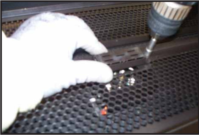
Figure 8.8 Removing Pilot Shield
