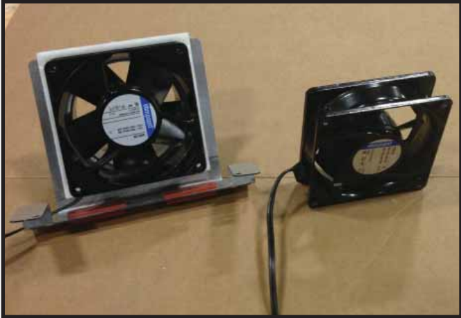
Figure 8.21. Proper Blower Mounting.
