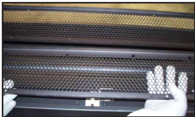
Figure 8.10 Lifting Base Pan Up and Out.
