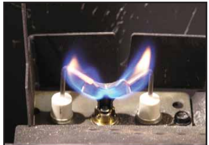
Figure 4.2 IPI Pilot Flame Patterns
