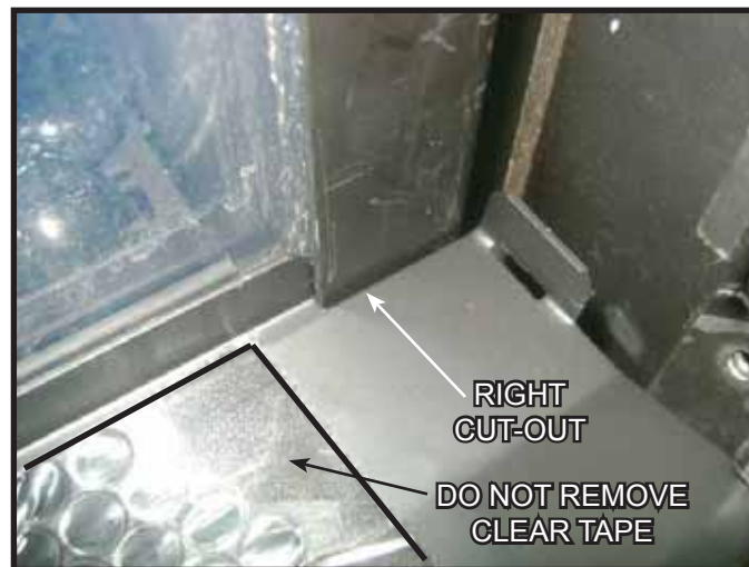
Figure 4.A.6. Front Access Media Tray
