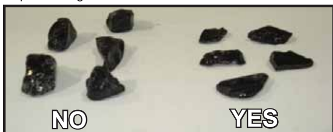
Figure 1. Selecting Flat Rock Media for Pilot Cover.
