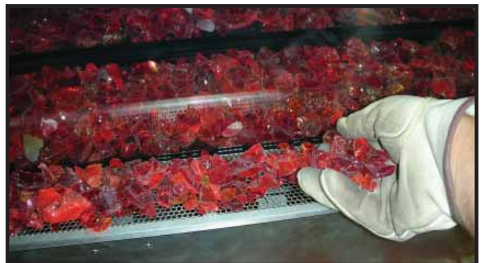
Figure 8. Placing Rock Media in Front Tray.
