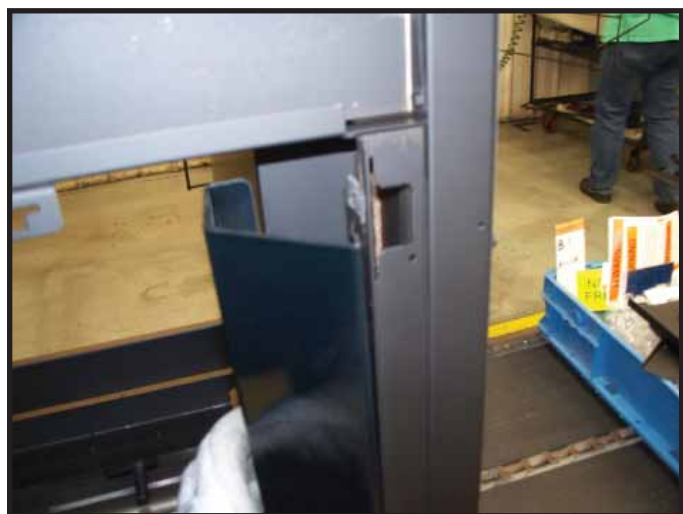
Figure 9. Install Corner Panel onto Clip.
