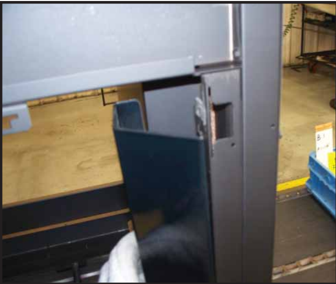
Figure 18. Installing Corner Panel onto Clip.
