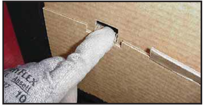
Figure 13.9 Securing Tabs Inside Front of Splatter Guard
