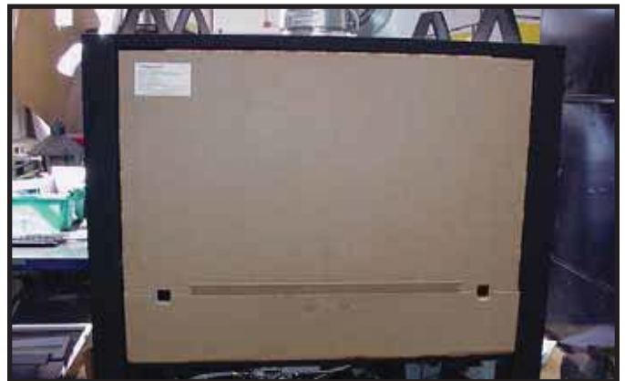
Figure 13.10 Splatter Guard with Lower Access Panel Open
