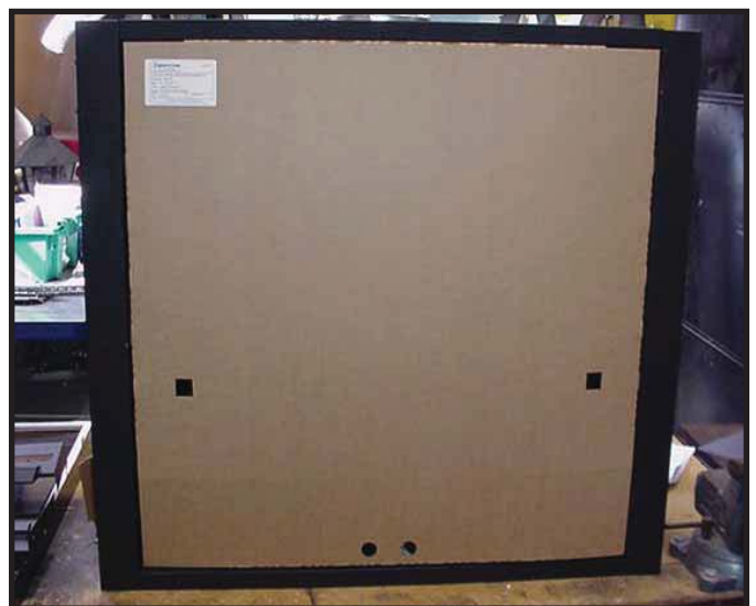
Figure 13.11 Splatter Guard with Lower Access Panel Closed
