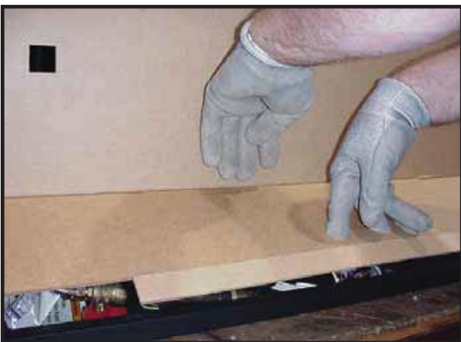
Figure 13.8 Opening Lower Access Panel
