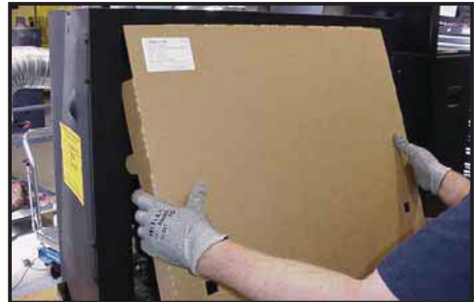
Figure 13.4 Installation of Splatter Guard
