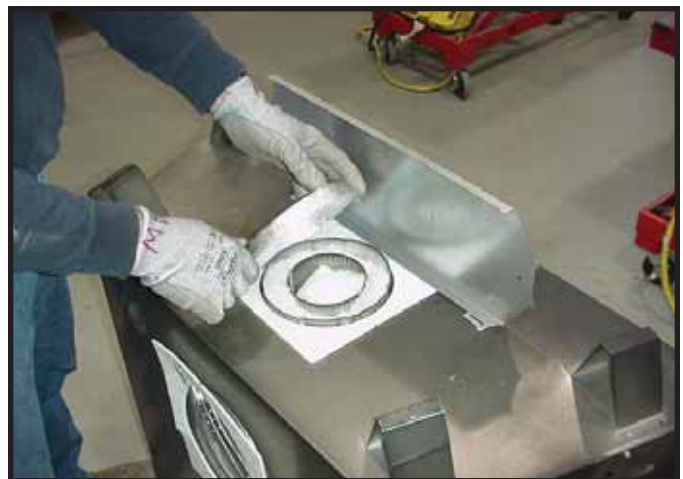
Figure 7.4 Remove the vent cap.
