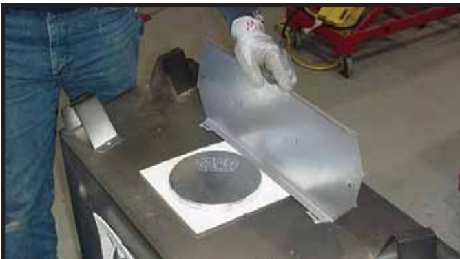
Figure 7.2 Rotate the top heat shield to the vertical position as shown above. The heat shield must remain in the vertical position.
