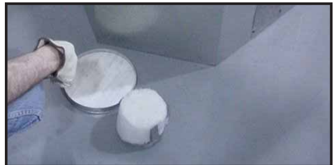
Figure 7.11 Discard the vent cap, remove and discard the insulation basket. Note: Once the vent cap has been removed it CANNOT be reattached.
